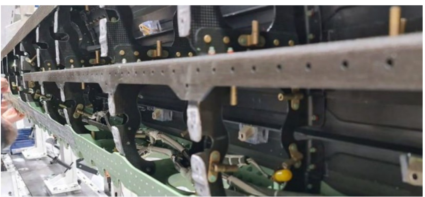
Integration of the high-voltage electrical harness on the wing of Lilium Jet MSN-1.
