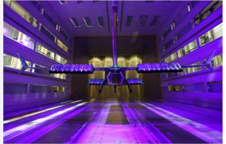
Successful wind tunnel testing at the DNW facility in Marknesse, Netherlands. The special lighting makes air flow attachment visible – indicated by the straight tufts of fabric on the aircraft surface.
