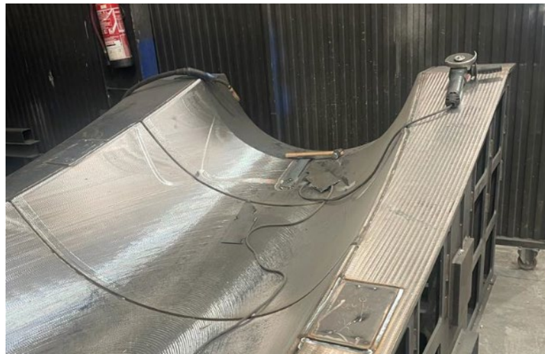
Layup mold for the bottom skin of the Lilium Jet fuselage. In order to manufacture the lightweight skin of the aircraft, composite material is laid up over the mold before being cured.
