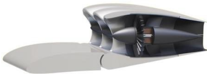
Picture illustrates a cross-section of our ducted fan, embedded in the flap of the jet's wing.
